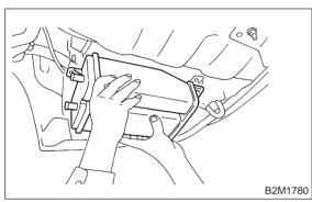
4) Disconnect connector from drain valve.
