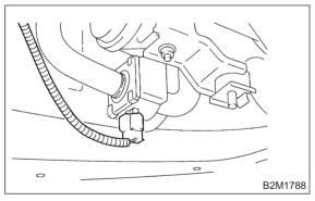
5) Disconnect evaporation hoses from drain valve.
