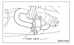
6) Remove bolt which installs air filter and drain valve brackets on body.
