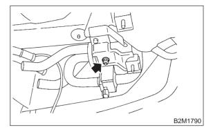
7) Move air filter to upper side, and remove drain valve with bracket.
