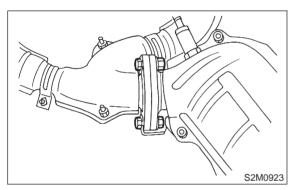
2) Install front and rear catalytic converter assembly.
