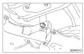
9) Separate front and rear catalytic converter assembly from front exhaust pipe.
