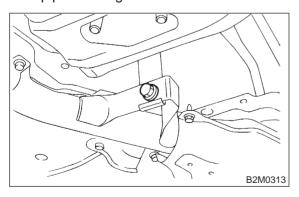
3) Install front exhaust pipe to cylinder heads.
