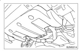
5) Disconnect rear oxygen sensor connector.
