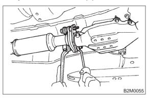
7) Remove front exhaust pipe from cylinder heads.
