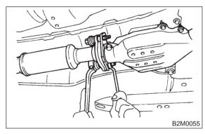
5) Tighten bolt which holds front and rear catalytic converter assembly to hanger bracket.
