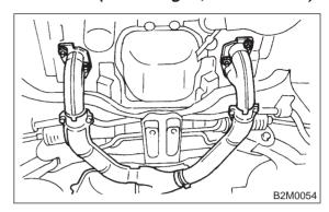
4) Install front and rear catalytic converter assembly to rear exhaust pipe.
