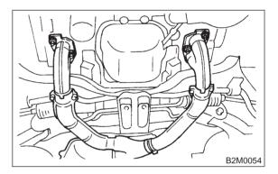
8) Remove front and rear catalytic converter assembly from hanger bracket.
