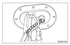
10) Remove main fuel level sensor from fuel pump assembly. <Ref. to 2-1 [W8A0].>
