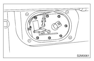
8) Take off fuel pump assembly from fuel tank.
