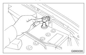
4) Disconnect connector from fuel pump.
