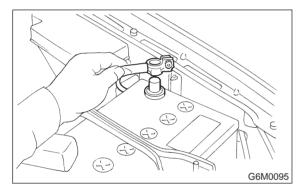
4) Disconnect connector from fuel pump.
