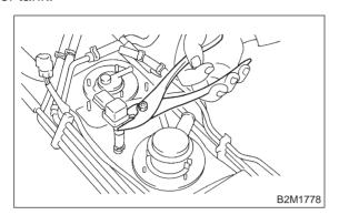
11) Disconnect pressure hose from fuel tank pressure sensor.
