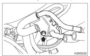
5) Disconnect connector from pressure control solenoid valve.
