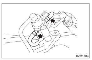
8) Remove pressure control solenoid valve from bracket.
