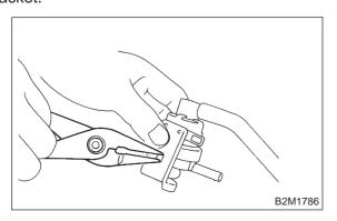
9) Disconnect vacuum hose from pressure control solenoid valve.
