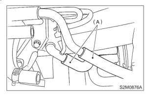
4) Remove bolt which installs pressure control solenoid valve holding bracket on body.
