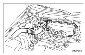
3) Remove air intake duct and air intake chamber. (Except 2200 cc California spec. vehicles) <Ref. to 2-7 [W18A0].>
