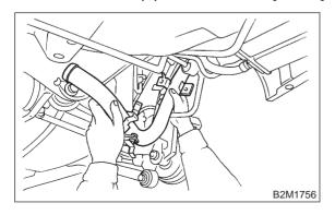
6) Disconnect evaporation hoses from shut valve.
