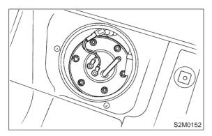
7) Remove sub fuel level sensor.
