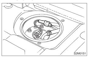
6) Remove bolts which install sub fuel level sensor on fuel tank.
