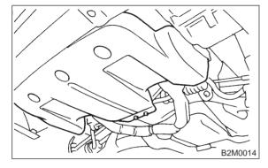
3) Fit vinyl tube to drain pipe.
