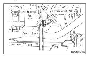
4) Loosen drain cock to drain engine coolant into container.
