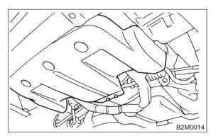
4) Disconnect connector of sub fan motor.
