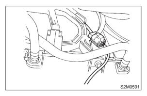
5) Detach ATF cooler hose attached to 2 clips under the radiator main fan shroud.
