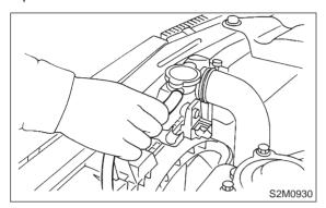
2) Remove bolts which install reservoir tank onto radiator main fan shroud.
