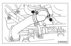
5) Install the thermostat in the intake manifold, and install the thermostat cover together with a gasket.
