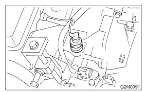
3) Remove oil pressure switch.
