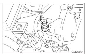
4) Install generator on bracket and temporary tighten installing bolts.
