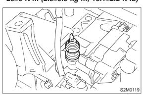
3) Connect terminal of oil pressure switch.
