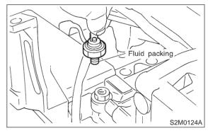
2) Install oil pressure switch onto engine block.
