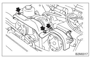
(3) Loosen lock bolt and slider bolt, and remove front side V-belt.
