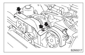
7) Connect connector and terminal to generator.
