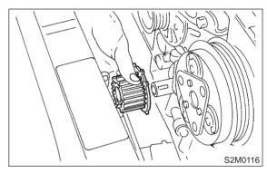
17) Remove bolts which install oil pump onto cylinder block.
