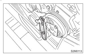
12) Remove crankshaft pulley by using ST. ST 49997700 CRANKSHAFT PULLEY WRENCH
