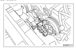
18) Remove oil pump by using flat bladed screw-driver.
