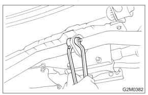
3) Install rear exhaust pipe to front catalytic converter.
