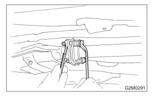
2) Separate rear exhaust pipe from muffler.
