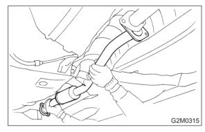
2) Install rear exhaust pipe to muffler.
