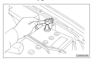
2) Disconnect connector from mass air flow sensor.
