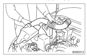
5) Disconnect connector from intake air temperature sensor.
