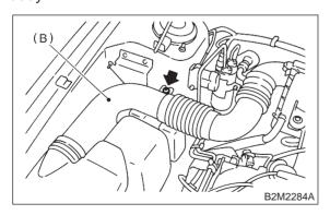
4) Remove air intake duct (A) and (B) as a unit.
