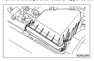
5) Remove air intake duct and air cleaner upper cover as a unit.
