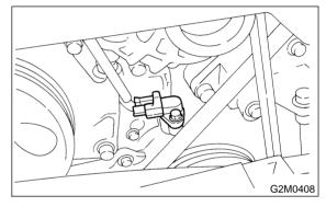
3) Remove crankshaft position sensor, and disconnect connector from it.
