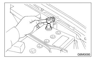
2) Remove bolt which install crankshaft position sensor to cylinder block.
