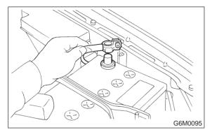
2) Remove bolt which installs air intake duct (A) on the front side of body.
