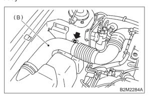
4) Remove air intake duct (A) and (B) as a unit.
