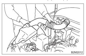
5) Disconnect connector from engine coolant temperature sensor.
