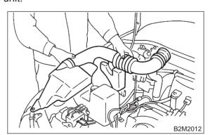
(2) Remove resonator chamber.
