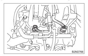
13) Remove bolts which install injector pipe to intake manifold.
