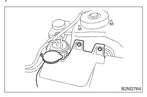
8) Move washer tank, and secure it away from working area.
