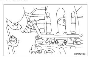
11) Pull up injector pipe, and remove fuel injector from intake manifold.
