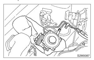
8) Remove band which holds engine harness to fuel injector pipe.
