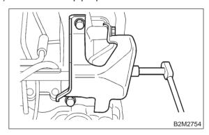
11) Remove band which holds engine harness to fuel injector pipe.
