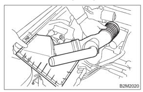
6) Remove spark plug cords from spark plugs (#1 and #3 cylinders).
