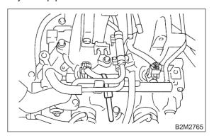
12) Disconnect connector from fuel injector.
