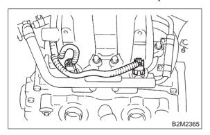
10) Remove bolts which install injector pipe to intake manifold.
