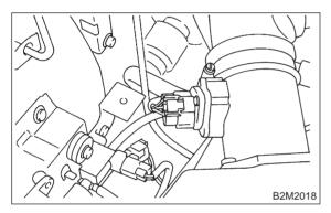
(2) Remove air intake duct and air cleaner upper cover as a unit, and remove air cleaner element. <Ref. to 2-7 [W1A0].>
