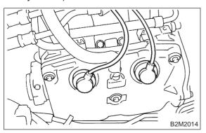
7) Remove power steering pump from bracket.
