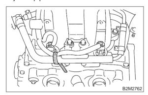
9) Disconnect connector from fuel injector.
