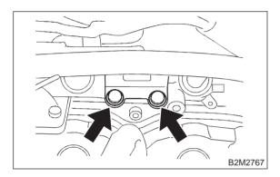
14) Pull up injector pipe, and remove fuel injector from intake manifold.
