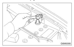
2) Disconnect connector from fuel pump relay.
