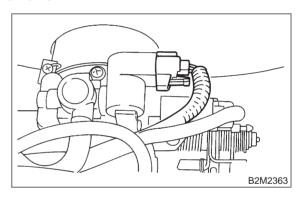
3) Disconnect air by-pass hose from idle air control solenoid valve.
