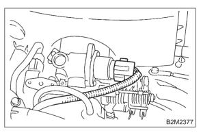
3) Remove idle air control solenoid valve from throttle body.
