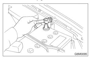
2) Disconnect connector from idle air control solenoid valve.
