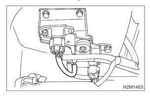
4) Remove pressure sensor from bracket.
