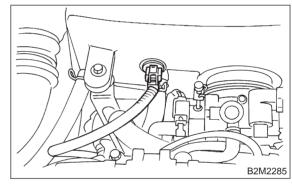
3) Remove intake air temperature sensor from air cleaner case.
