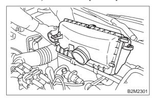
4) Install air cleaner assembly. (California spec. vehicles only) <Ref. to 2-7 [W1A0].>
