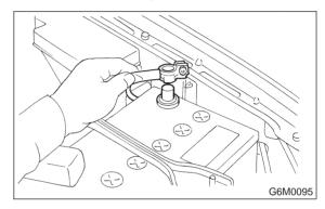
2) Remove idle air control solenoid valve. <Ref. to 2-7 [W12A1].>
