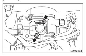
3) Disconnect connector from intake manifold pressure sensor.
