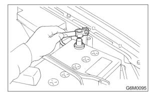
4) Disconnect connector from mass air flow sensor.
