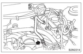
19) Remove air cleaner case stay RH and engine harness bracket, and disconnect engine harness connectors from bulkhead harness connectors.20) Pull out engine harness connector from bracket.
