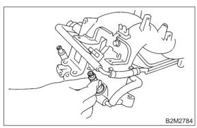
13) Loosen clamp which holds front left side fuel hose to injector pipe.
