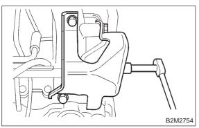
16) Disconnect spark plug cords from ignition coil and ignitor assembly.
