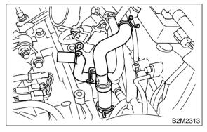
13) Connect spark plug cords to ignition coil and ignitor assembly.
