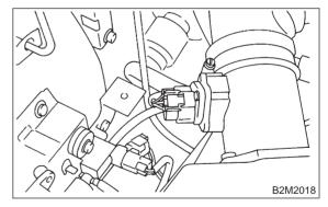
5) Loosen clamp which connects air intake chamber to throttle body.
