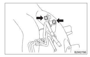
15) Remove two bolts which install fuel pipes on intake manifold.
