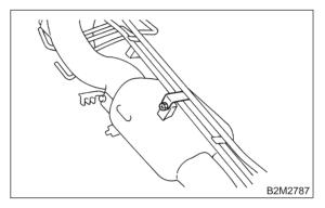
16) Remove fuel injector pipe.
