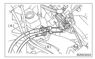
13) Disconnect vacuum hoses from pressure sources switching solenoid valve.
