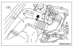
21) Tighten bolts which install air cleaner case to stays.
