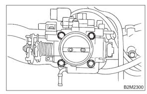
7) Disconnect connectors from fuel injectors, and purge control solenoid valve.
