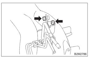
14) Remove two bolts which install fuel pipes on intake manifold.
