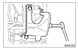
15) Install power steering pump on bracket.(1) Tighten bolts which install power steering pump on bracket.
