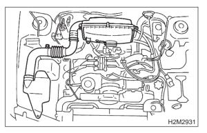
19) Tighten bolt which installs air intake duct (A) on the front side of body.
