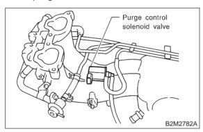
9) Install engine harness onto intake manifold.10) Connect connectors to fuel injectors and purge control solenoid valve.
