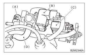
15) Install ignition coil and ignitor assembly.
