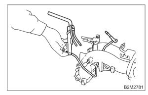
17) Remove fuel pipes, etc. from intake manifold.
