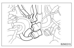
21) Disconnect connectors from engine coolant temperature sensor.
