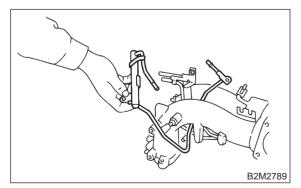
3) Tighten two bolts which install fuel pipes on intake manifold.
