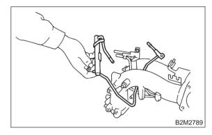
16) Remove fuel pipes, etc. from intake manifold.
