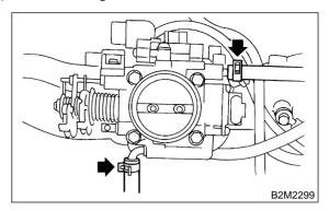
12) Connect PCV hose and pressure regulator vacuum hose to intake manifold.
