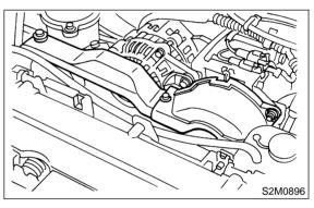
(2) Loosen lock bolt and slider bolt, and remove power steering pump drive V-belt.
