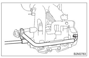
8) Install purge control solenoid valve.
