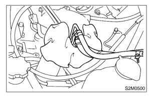
28) Remove bolts which hold intake manifold onto cylinder heads.
