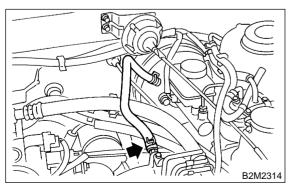
11) Connect engine coolant hose to throttle body.
