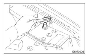
4) Disconnect connector from intake air temperature sensor.
