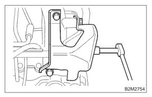
15) Disconnect spark plug cords from ignition coil and ignitor assembly.
