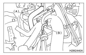
12) Connect spark plug cords to ignition coil and ignitor assembly.
