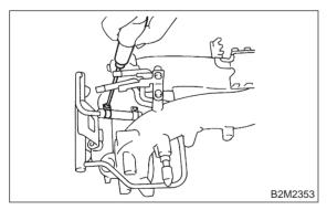
13) Remove bolts which hold fuel pipes on the left side of intake manifold.
