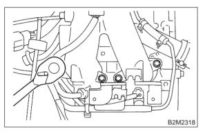
28) Remove intake manifold.
