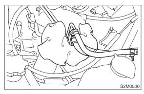
3) Connect connector to oil pressure switch.
