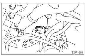
8) Hold engine harness connector onto bracket.9) Install air cleaner case stay RH and engine harness bracket, and connect engine harness con-
