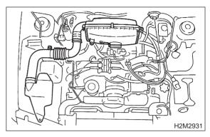
11) Disconnect accelerator cable (A).
