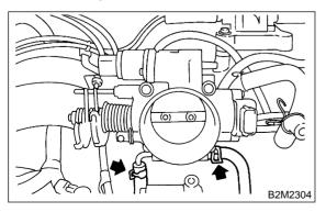
11) Connect PCV hose (A) and vacuum hose (B) to intake manifold.
