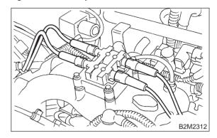
17) Disconnect PCV hose (A) and pressure regulator vacuum hose (B) from intake manifold.18) Disconnect vacuum hose (C) to cruise control diaphragm. (With cruise control models)
