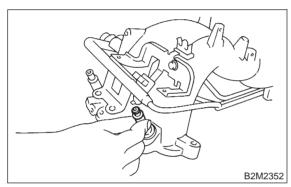
12) Loosen clamp which holds front left side fuel hose to injector pipe.
