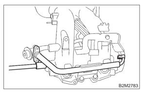
8) Install purge control solenoid valve.
