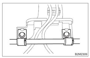
(5) Remove bolts which install power steering pump to bracket.
