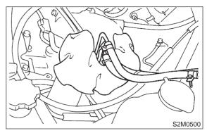
3) Connect connector to oil pressure switch.
