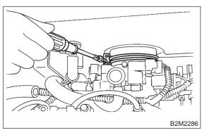
9) Disconnect blow-by hose from air cleaner case.10) Remove air intake duct (A), (B) and air cleaner assembly as a unit.
