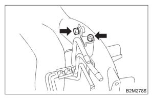
5) Connect left side fuel hose to injector pipe, and tighten clamp screw.
