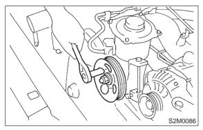
(2) Install power steering pipe brackets on the right side of intake manifold.
