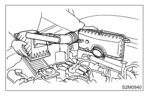
11) Disconnect accelerator cable (A).
