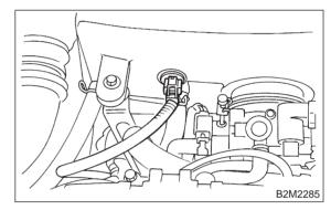
23) Connect connector to fuel pump relay.
