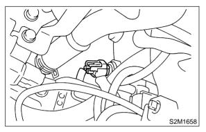
8) Install air intake chamber stay RH and engine harness bracket, and connect engine harness connectors to bulkhead connectors.
