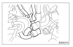
22) Disconnect connectors from engine coolant temperature sensor.
