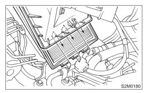
18) Tighten bolts which install air intake chamber to stays.
