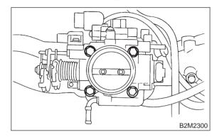
13) Connect connectors to throttle position sensor (A), idle air control solenoid valve (B) and intake manifold pressure sensor (C).
