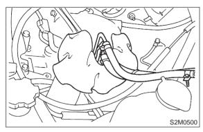
27) Remove eight bolts which hold intake manifold onto cylinder heads.
