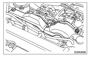
(6) Install resonator chamber.
