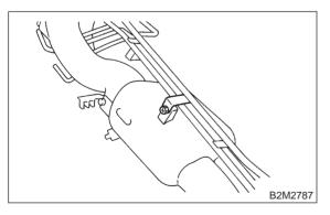
4) Tighten two bolts which install fuel pipes on the left side of intake manifold.
