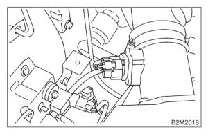
20) Connect connector to fuel pump relay.
