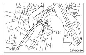
19) Disconnect engine coolant hose from throttle body.
