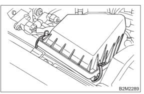
7) Remove bolts which install air intake chamber on stays.
