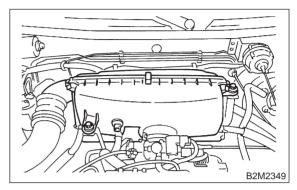
22) Connect connector to intake air temperature sensor.
