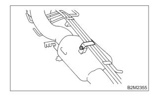
15) Remove fuel injector pipe.
