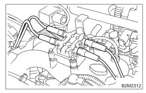
16) Disconnect PCV hose assembly from intake manifold.
