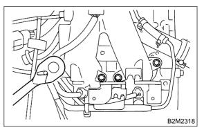
29) Remove intake manifold.
