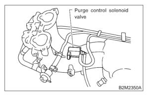
9) Install engine harness onto intake manifold.
