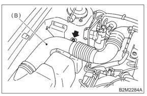
7) Remove bolts which install air cleaner case on stays.
