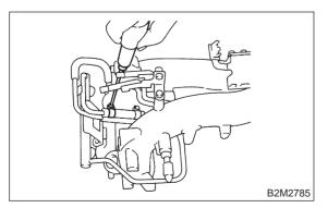
14) Remove bolts which hold fuel pipes on the left side of intake manifold.
