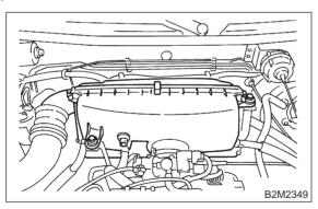
8) Loosen clamp which connects air intake chamber to throttle body.
