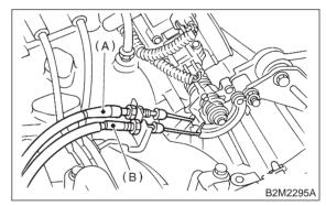
13) Remove power steering pump from bracket.(1) Remove resonator chamber.
