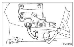
4) Remove pressure sensor from bracket.
