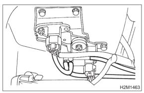
4) Remove pressure sources switching solenoid valve from bracket.
