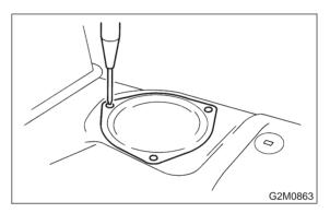
4) Disconnect connector from fuel sub meter, and disconnect jet pump hose.
