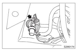
3) Disconnect hoses from roll over valve, and remove it from bracket.
