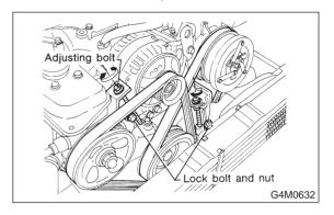
6) Check drive belt tension and adjust it if necessary by changing alternator position and/or idler pulley position.
