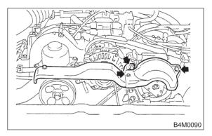
2) Check that clearance between drive plate and pulley over the entire perimeter is within specifications.
