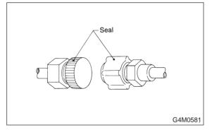
2) Visually inspect the O-ring surface, the O-ring mating surface, the threads and the connection points. If a defective part is found, replace it. The O-ring must sit square against the tube bead. If necessary, slide the O-ring into proper position with clean hands.
