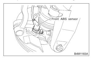
5) Remove front disc brake caliper and disc rotor from housing after removing front tire.
