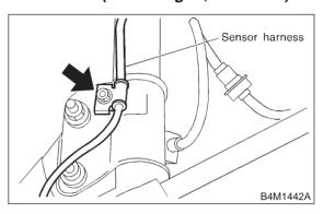
5) Place a thickness gauge between ABS sensor's pole piece and tone wheel's tooth face. After standard clearance is obtained over the entire perimeter, tighten ABS sensor on housing to specified torque.
