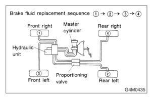
3) Slowly depress the brake pedal and keep it depressed. Then, open the air bleeder to discharge air together with the fluid.
