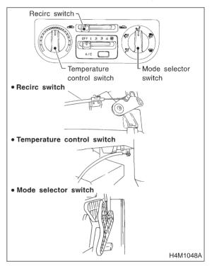
4) Remove center panel from instrument panel then disconnect connectors.
