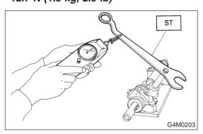
Sliding resistance: Right-turn steering; 304 N (31 kg, 68 lb) or less
