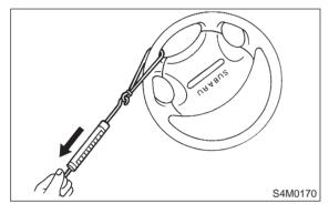
2) Measurement of folding torque of universal joint is as shown in the figures.
