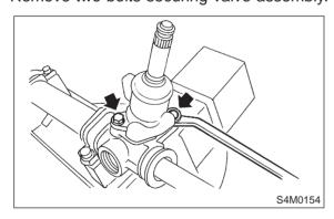
2) Carefully draw out input shaft and remove valve assembly.
