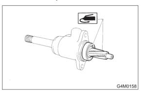
4) Install gasket on valve assembly. Insert valve assembly into place while facing rack teeth toward pinion.
