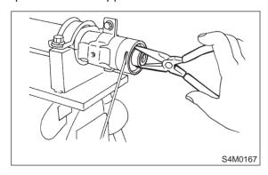
8) Fit mounting rubber onto rack housing.
