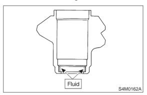
3) Attach ST2 to ST1, and press oil seal into place using a press.
