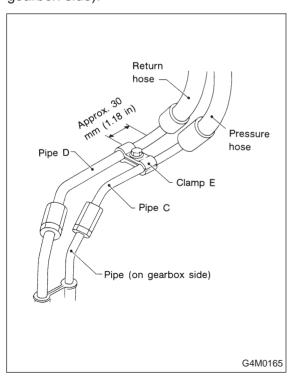
4) Temporarily install clamp E on pipes C and D.
