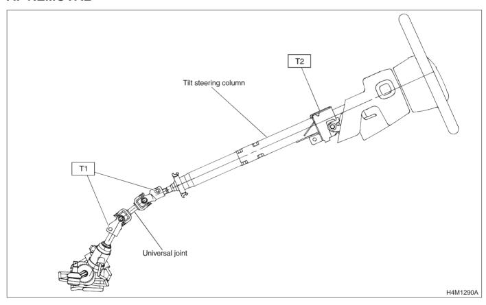
Tightening torque: N·m (kg-m, ft-lb) T1: 24±3 (2.4±0.3, 17.4±2.2) T2: 25±5 (2.5±0.5, 18.1±3.6)
