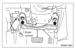
7) Align center of roll connector. (with airbag model) <Ref. to 5-5 [W6B1].>
