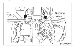
10) Pull out steering shaft assembly from hole on toe board.
