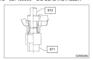
9) Apply sufficient grease to oil seal lip.
