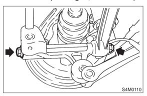
4) Connect rear housing assembly to trailing link assembly.
