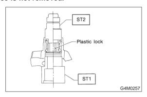
4) Using plier, install snap ring.
