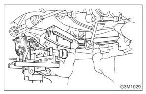
2) Insert DOJ of rear drive shaft into rear differential.
