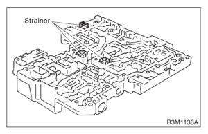
5) Install lower separate plate to lower valve body.
