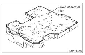
6) Temporarily assemble valve body.
