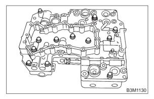
4) Separate the control valve body.
