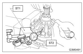
5) Using ST, install taper roller bearing. ST 398487700 DRIFT
