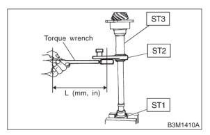
5) Measure the starting torque of the bearing. Make sure the starting torque is within the specified range. If out of the allowable range, replace the roller bearing.
