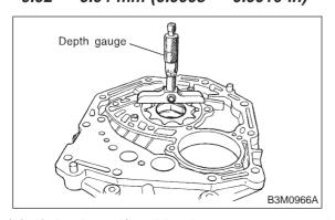
(3) If depth and/or side clearances are outside specifications, replace rotor assembly.
