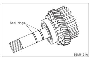
2) Using ST, remove the ball bearing. ST 498077600 REMOVER
