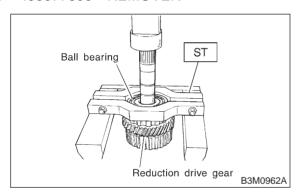
3) Using a press, remove the reduction drive gear.
