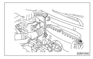
2) Remove air intake duct and cleaner case. (2200 cc California spec. vehicles) <Ref. to 2-7 [W1A0].> and <Ref. to 2-7 [W18A0].>
