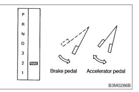
6) When the engine speed is stabilized, read that speed quickly and release the accelerator pedal.7) Shift the select lever to Neutral, and cool down the engine by idling it for more than one minute.8) Record the stall speed.
