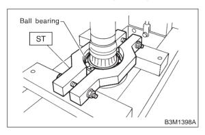
2) Install ball bearing to center differential assembly.
