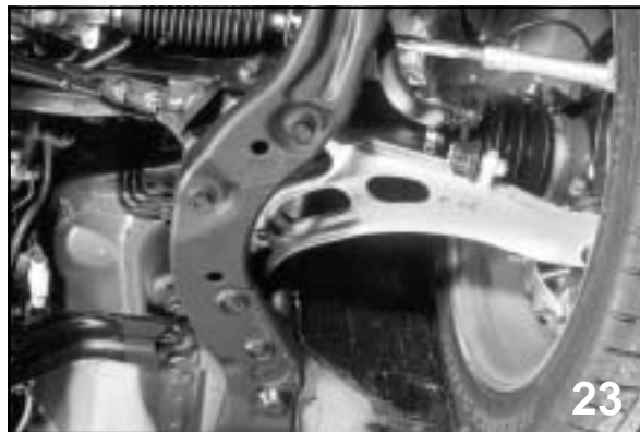
Front suspension with aluminum front transverse link
