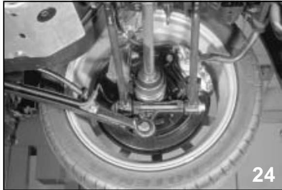
Rear suspension with ball joint support on stabilizer bar link
